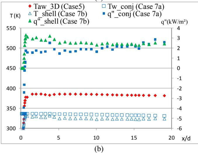
Figure 9 Heat flux, wall temperatures from 3D Cases (a) Cases 6.1, 6.2 and 6.3 (b) Cases 7a and 7b.  $T_{aw}$  along the centerline through the center of the hole from the 3D baseline case (Case5) and 2D baseline case (Case1) also included for comparison. Heat flux plotted on secondary axis on the right.
