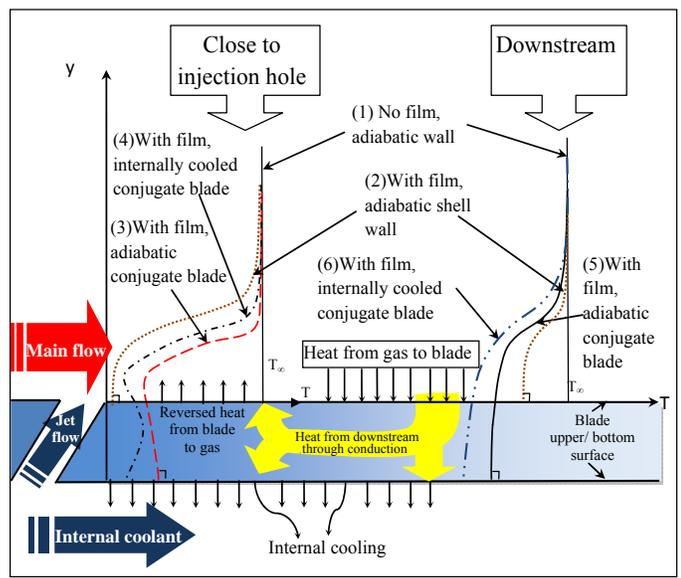
**Figure 1** Qualitatively temperature profiles of a typical internally and film cooled blade at two locations: one near the injection hole region with potentially reversed heat transfer and the other located further downstream. The axial heat conduction transfer is small and the size of reversed heat flux arrowhead is enlarged for illustration purpose.
