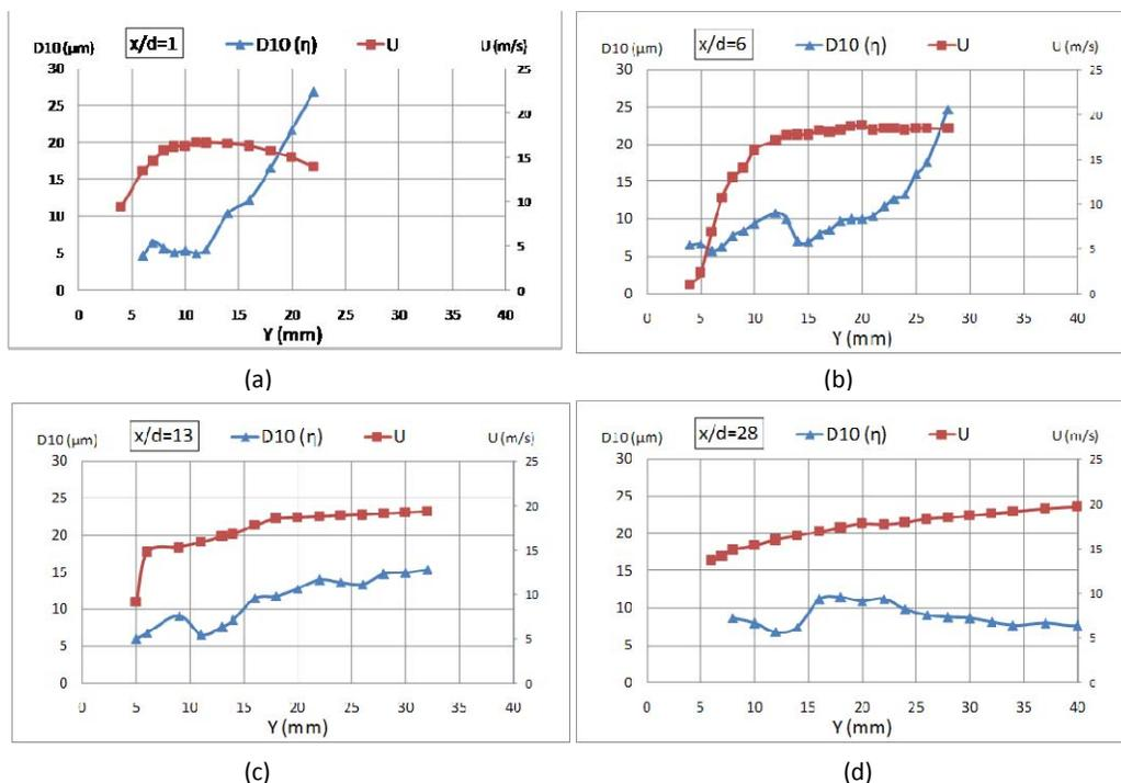
Figure 10 Particle size distribution (plotted on Y-coordinate on the left) and the droplets mean velocity (plotted on Y-coordinate on the right) as a function of Y locations at (a)  $X/D=1$  (b)  $X/D=6$  (c)  $X/D=13$  (d)  $X/D=28$
