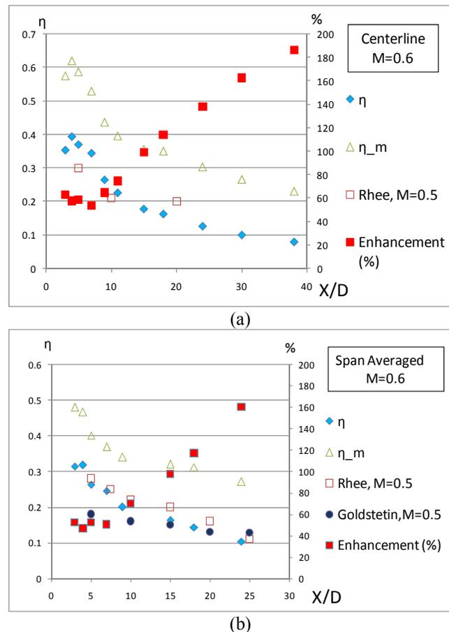
**Figure 3 Comparison of present adiabatic cooling effectiveness (left coordinate) and net enhancement (right coordinate) with the experimental data from Goldstein et al. and Rhee et al. (a) M=0.6, centerline data (b) M=0.6, spanwise averaged data**
