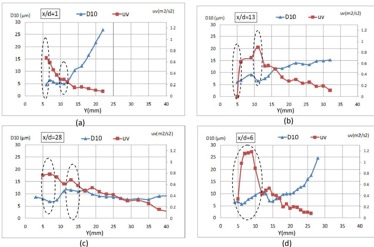
**Figure 9 (Case 2, M=0.6) Droplet size distribution (plotted on Y-coordinate on the left) and Reynolds Stress distribution (plotted on Y-coordinate on the right) as a function of Y-locations at (a) X/D=1 (b) X/D=6 (c) X/D=13 (d) X/D=28**
