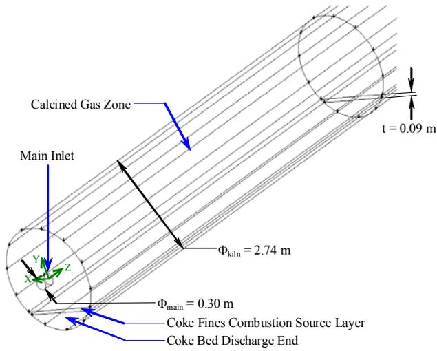
**Fig. 5 Detailed view of calcined coke zone near the discharge end**
