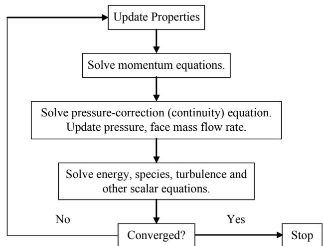
Fig. 11 Flow chart for segregated solver
