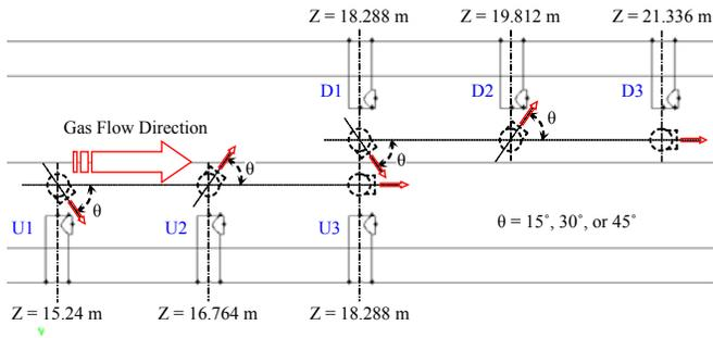
**Figure 13 Tertiary air injector locations and labeling**
