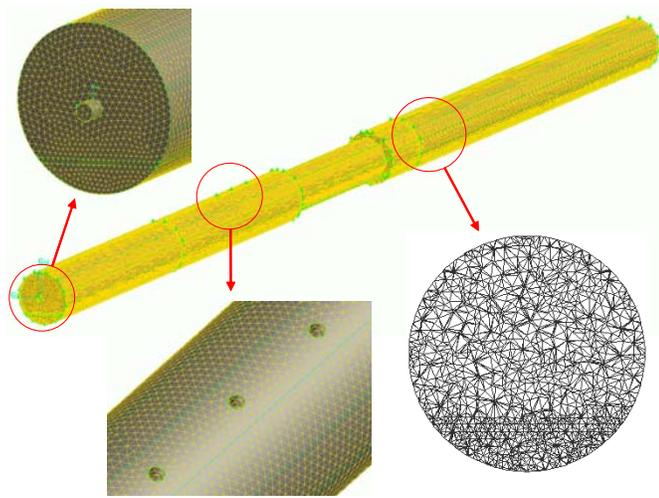
Fig. 10 Meshed geometry for the rotary calcining kiln
