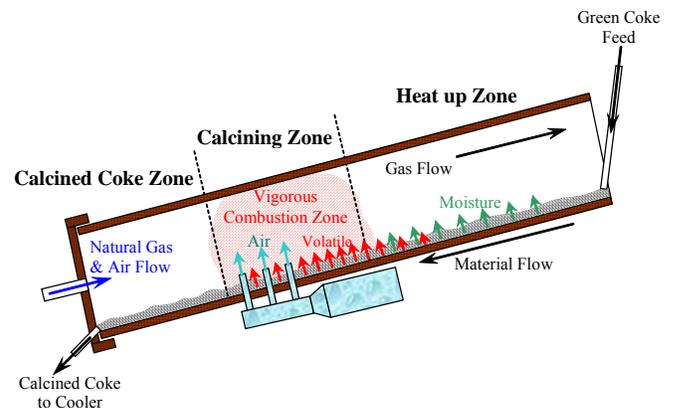
**Fig. 3 Petroleum coke calcination with tertiary air**
