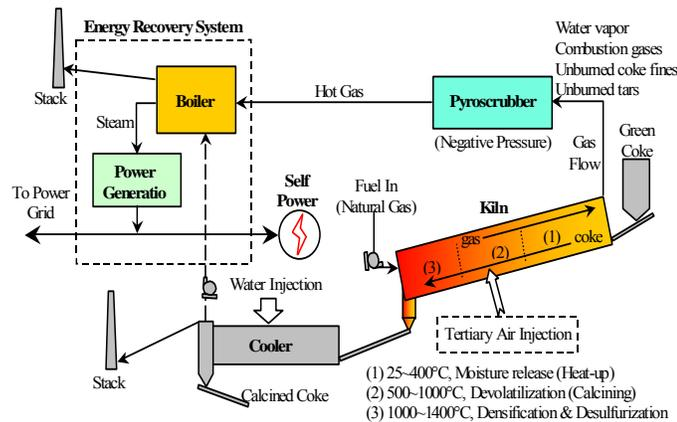
**Fig. 1 Schematic of calcining process for petroleum coke**
