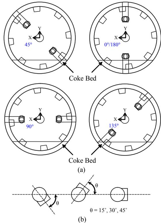
**Fig. 9 (a) Relative coke bed and tertiary air inlet position (rotational angles) (b) there different tertiary air injection angles**
