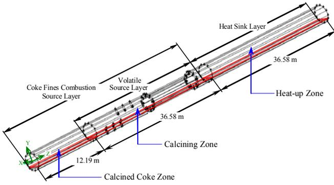
**Fig. 4 A 3-D view of the simulated calcining rotary kiln**
