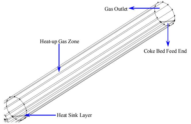
**Fig. 7 Close-up view of the heat-up zone**
