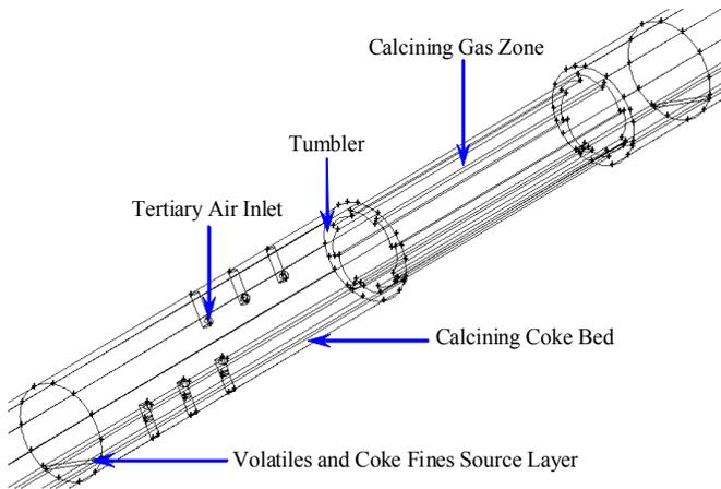
**Fig. 6 Detailed view of calcining coke zone including tertiary air injectors and tumblers**
