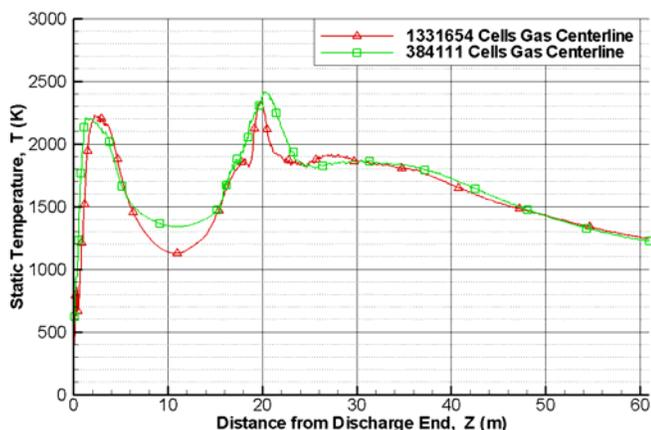
Fig. 12 Gas centerline static temperature for various cell numbers
