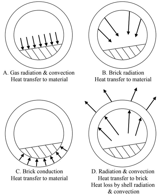
**Fig. 2 Heat transfer mechanism in a rotary kiln [1]**
