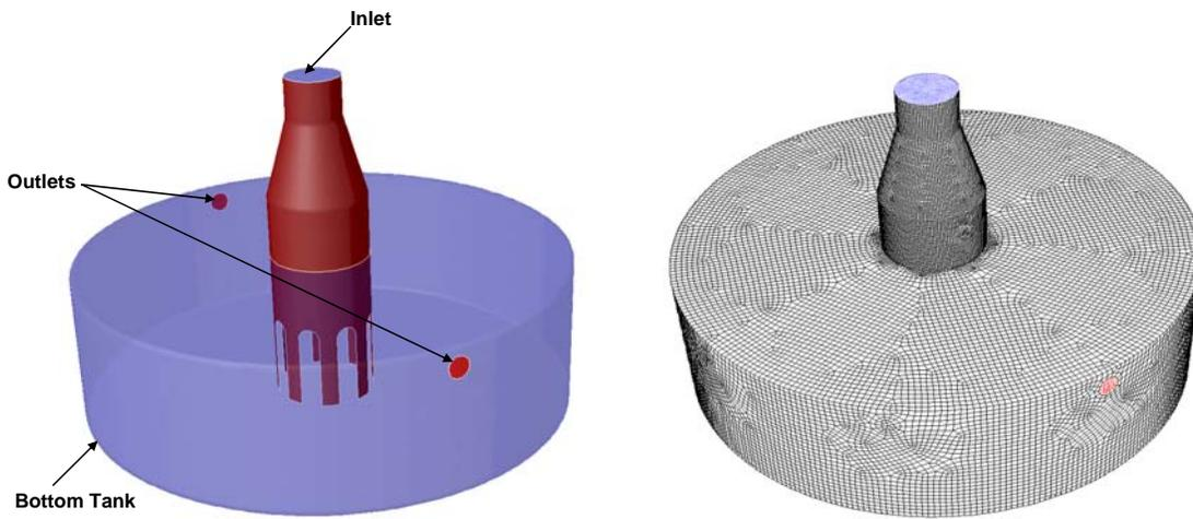
**Fig. 2 Geometry, boundary conditions and meshed computational domain of the quench section of the ITRI Gasifier**
