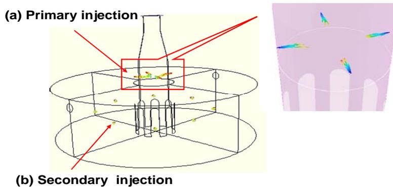
**Fig. 3 Locations of water injections: (a) the primary injection consisting of two pairs of opposing jets and (b) the secondary injection consisting of eight injectors spraying downward against the up moving flow.**
