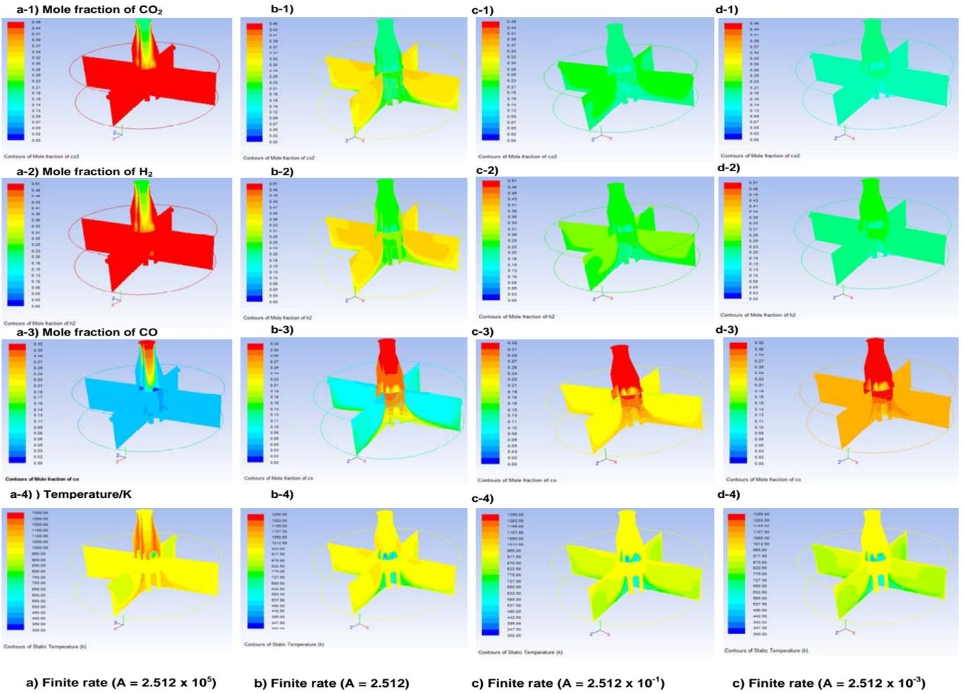
**Fig. 4** Variation of Temperature and syngas composition by changing the A value of Wade’s rate with the primary water injection. Faster rates produce more H<sub>2</sub> and CO<sub>2</sub>, lower CO, and higher temperature.
