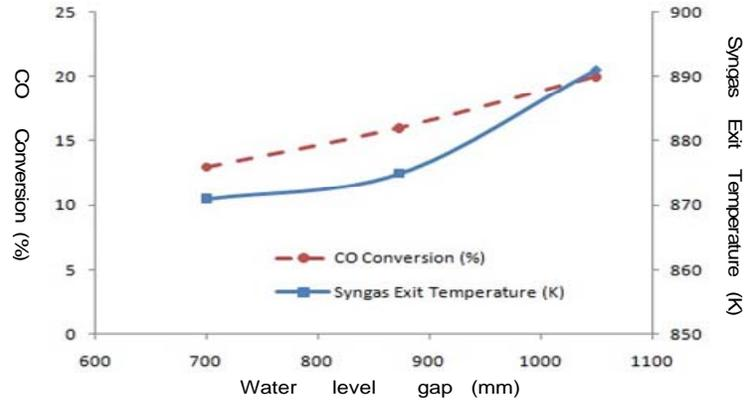
**Fig. 9 Effect of water level gap on WGS and syngas temperature using reaction rate  $A = 0.2512$   $E = 1.325 \times 10^5$  J/kmol**
