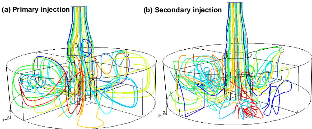
**Fig. 6 Syngas pathline for primary and secondary injection cases.**
