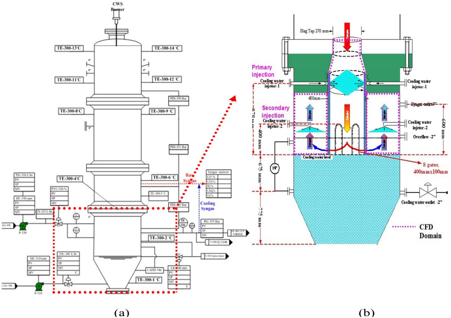
**Fig. 1 (a) Schematic diagram of ITRI downdraft coal slurry-fed gasifier (b) gasifier's quench section showing locations of water injections: primary at the inlet and secondary in the outer annular.**
