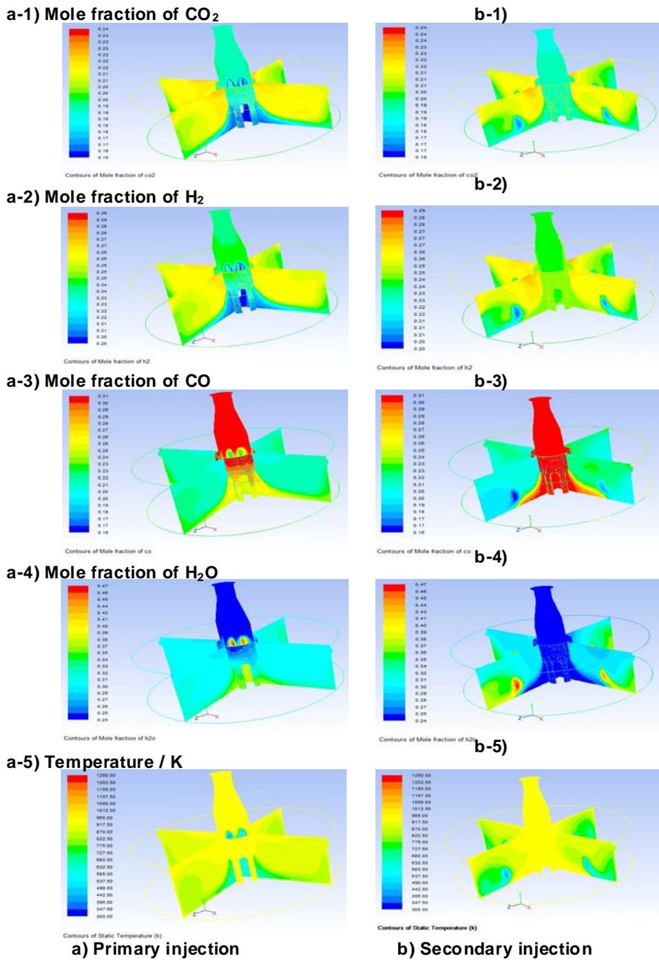
**Fig. 7 Distributions of temperature and various species on two selected planes for primary and secondary injection cases using reaction rate  $A = 0.2512$   $E = 1.325 \times 10^5$  J/kmol**
