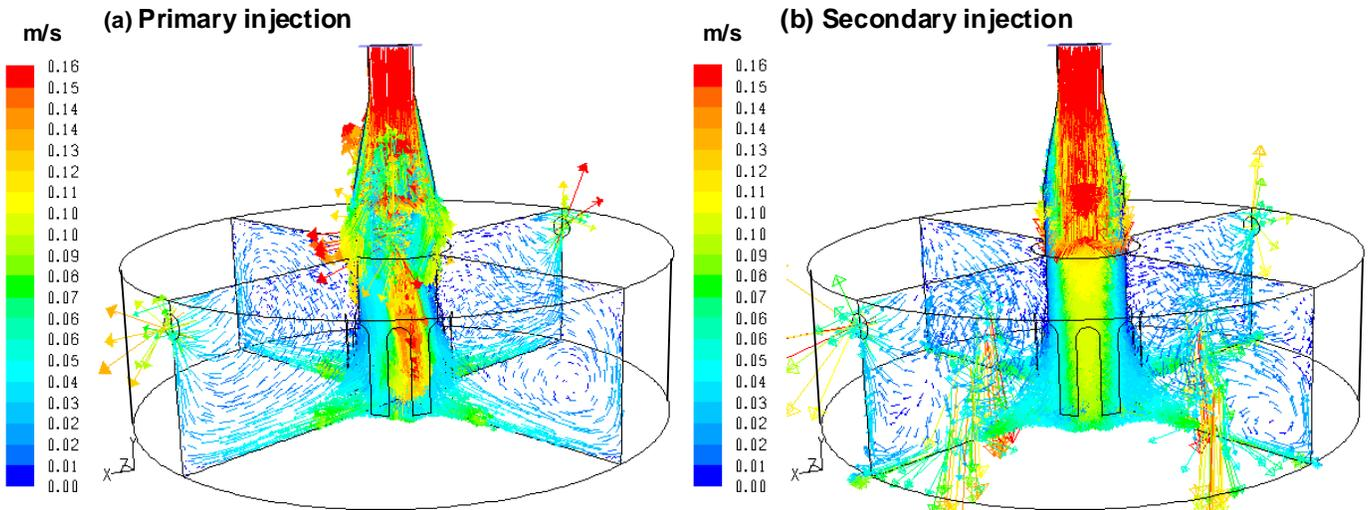
**Fig. 5 Velocity vector fields on two selected planes for primary and secondary injection cases, respectively**
