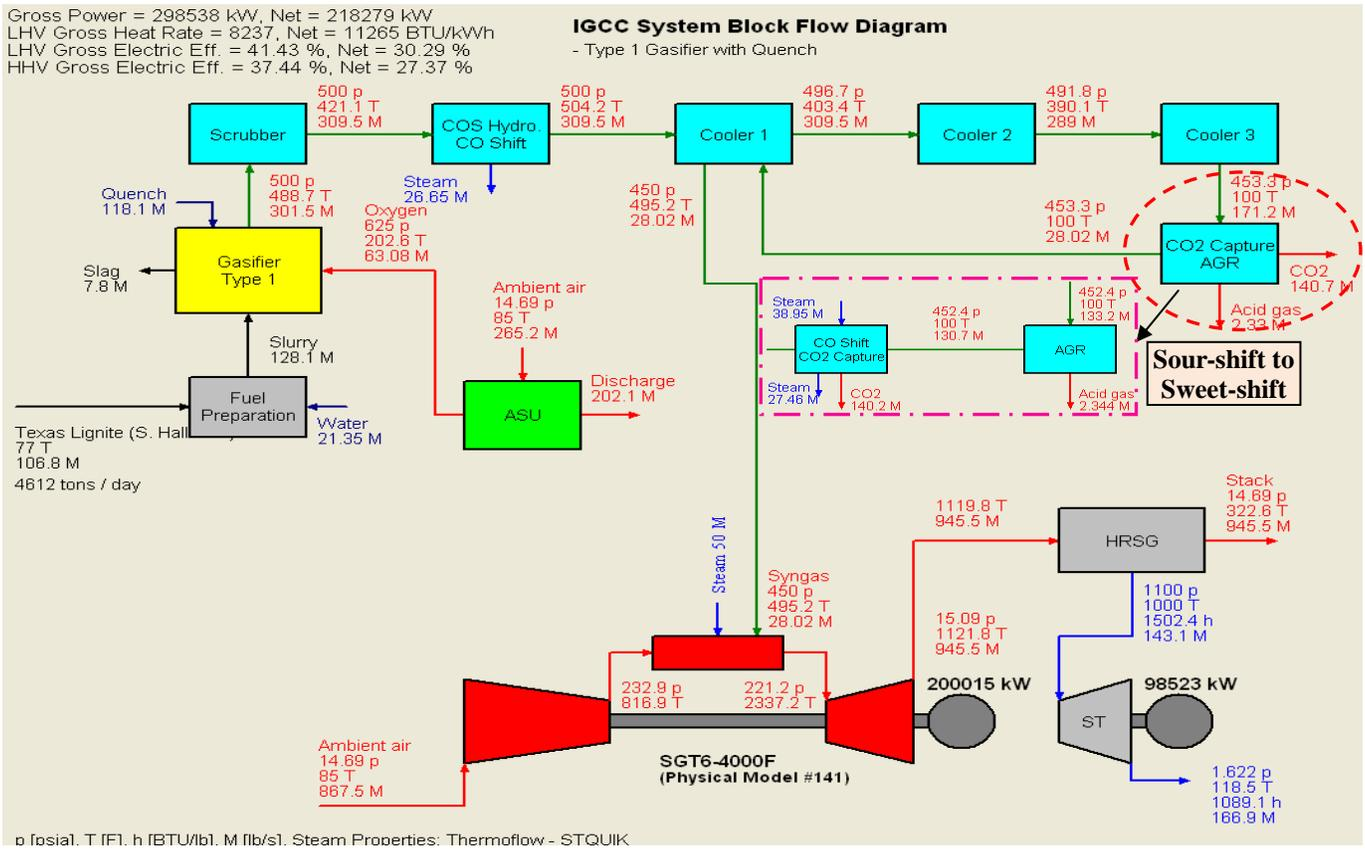
Figure 1 Overall plant layout with sour-shift with no biomass and subcritical steam. For sweet shift, the red dashed circle is replaced by the pink dashed box.
