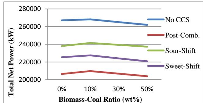
Figure 9 Total Net Power for supercritical plants
