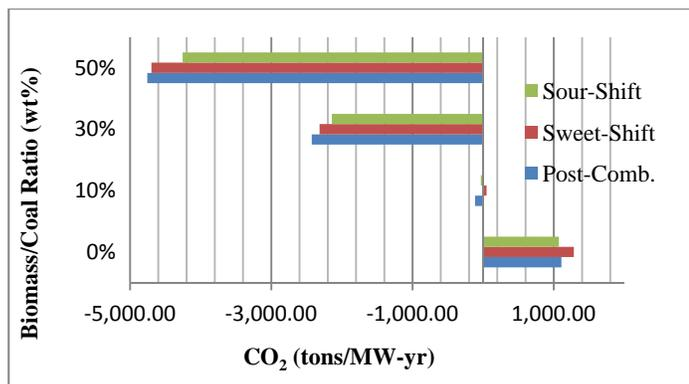
Figure 7 Effective CO<sub>2</sub> for subcritical plants with CCS
