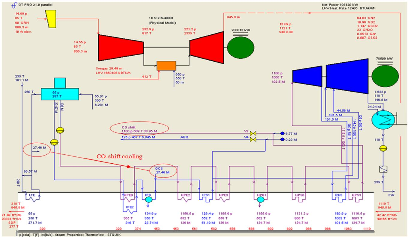
Figure 6 Steam cycle for sweet-shift CCS with CO-shift steam and cooling steam circled
