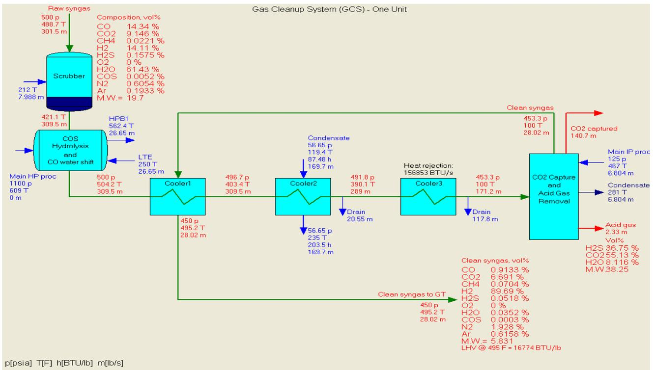
Figure 2 Pre-combustion CCS cleanup system with sour-shift
