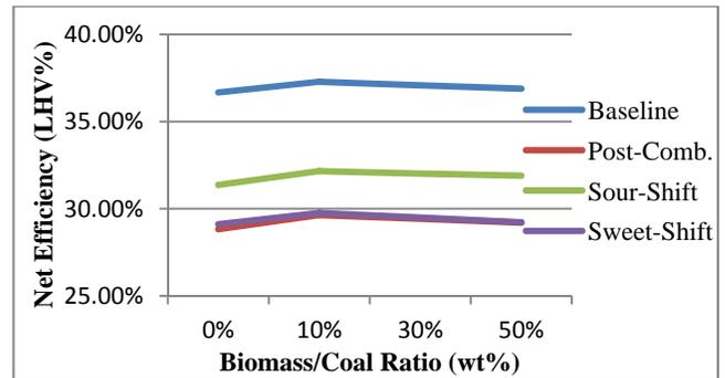
Figure 8 Efficiency for supercritical plants
