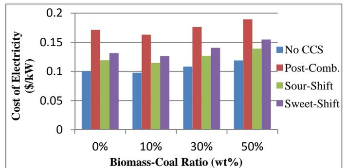
Figure 10 Cost of Electricity for subcritical plants
