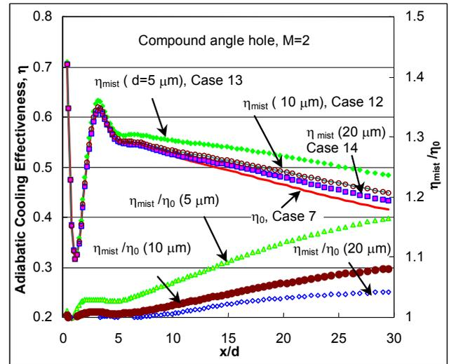
Figure 11 Effect of droplet size on mist cooling effectiveness (along the centerline of compound-angle hole cases 12 ~14)
