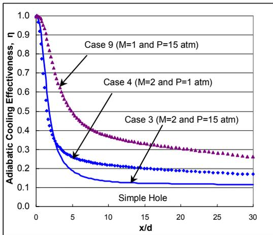
Figure 6 Effect of blowing ratio on a simple round hole adiabatic cooling effectiveness at elevated operating conditions
