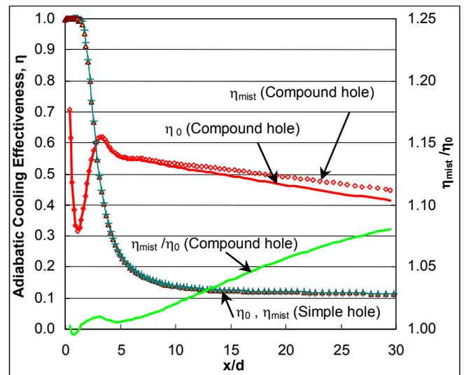
Figure 9 Enhancement of mist on film cooling along the centerline under the gas turbine operating conditions
