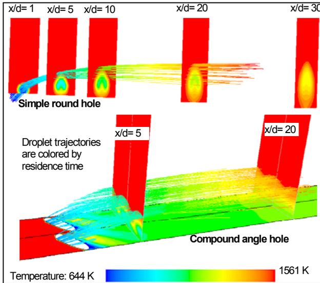
(a) Water droplet trajectories of simple and compound angle holes at 15 atm and 1561K. Droplets move away from the wall and the coolant flow and are shown on top of the coolant-affected area, so mist does not effectively enhance  $\eta$  under the elevated operating conditions.
