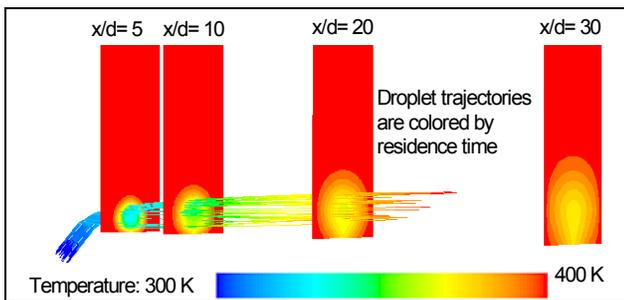
(b) Simple hole at low T, V and P conditions [22]
