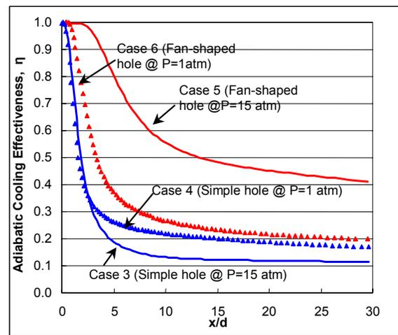
Figure 4 Effect of elevated operating conditions on adiabatic cooling effectiveness of 3-D film holes
