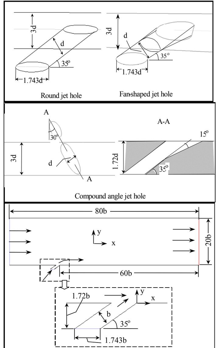
Figure 1 Computational domain and film hole configurations
