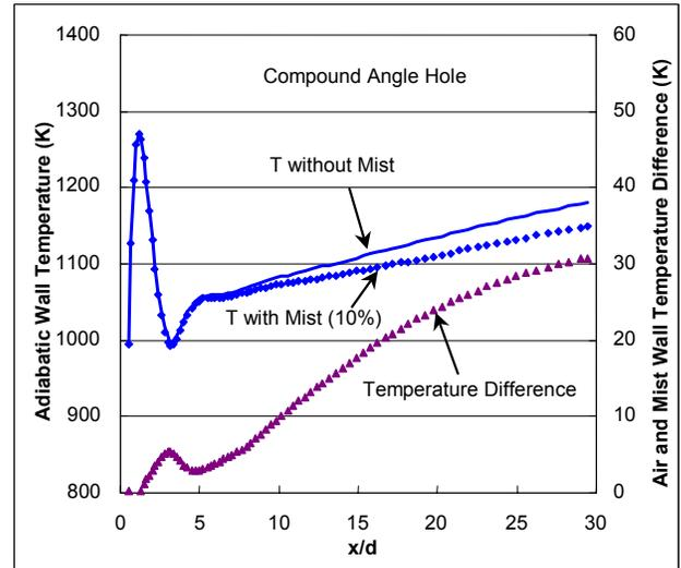
Figure 13 Adiabatic wall temperature distribution and reduction along the central line of compound-angle hole Case 12.
