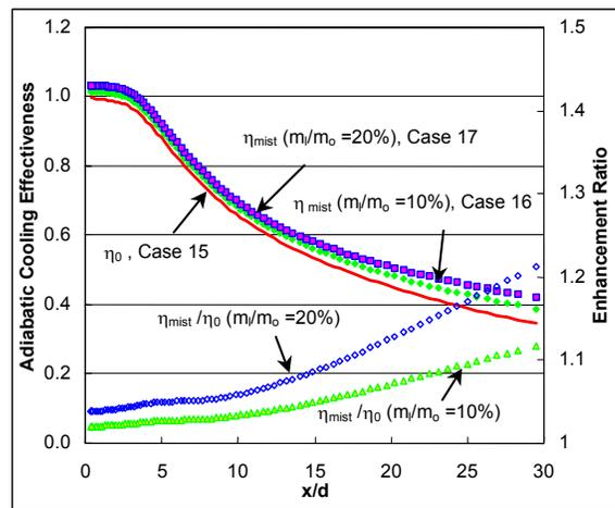
Figure 12 Effect of mist concentration on adiabatic cooling effectiveness (along the centerline of the fan-shaped hole cases 15, 16, and 17 with the blowing ratio  $M=1$ )
