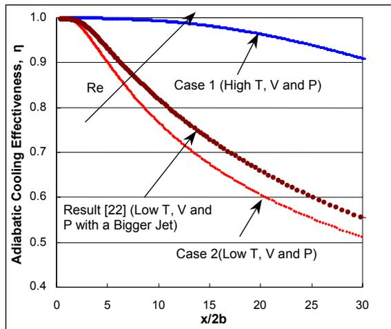
Figure 3 Comparison of slot jet adiabatic cooling effectiveness between low and elevated GT operating conditions
