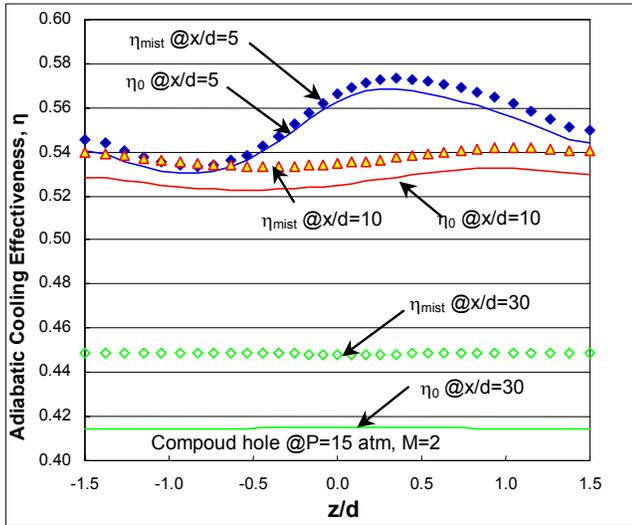
Figure 10 Distribution of adiabatic cooling effectiveness in spanwise direction (Compound angle hole, Case 12)
