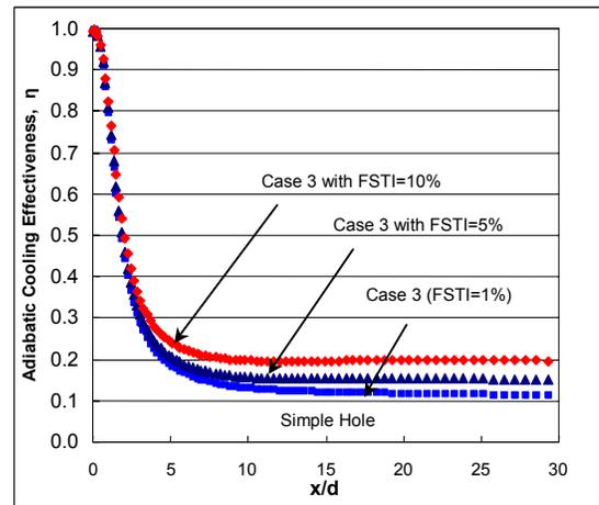
Figure 7 Effect of FSTI on a simple round hole adiabatic cooling effectiveness at 15 atm and 1561K.
