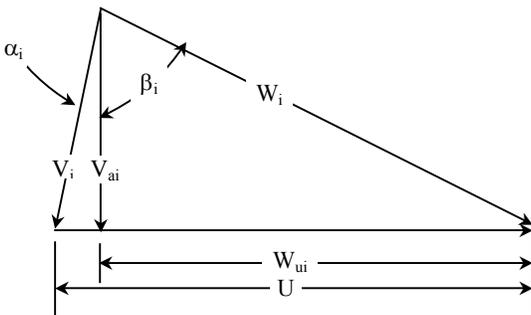
**Figure 5 Velocity Diagram at rotor inlet**
