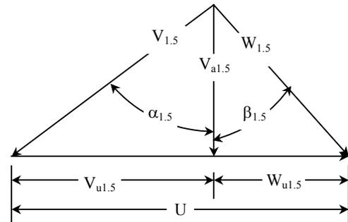
Figure 4 Velocity Diagram at rotor exit
