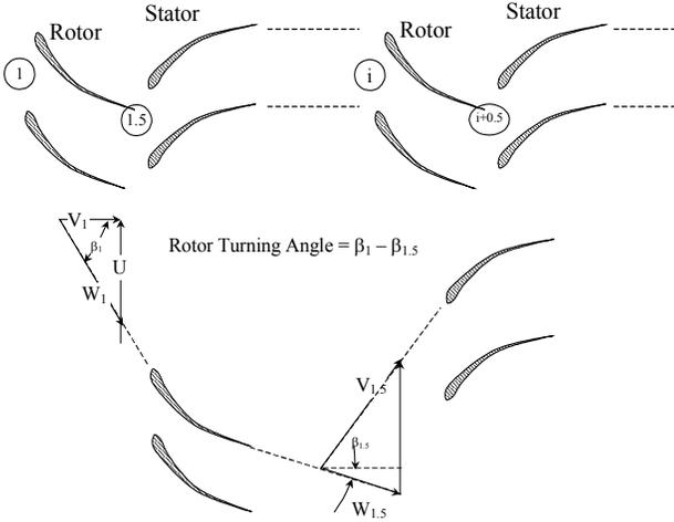
Figure 2 Rotor-Stator Staging
