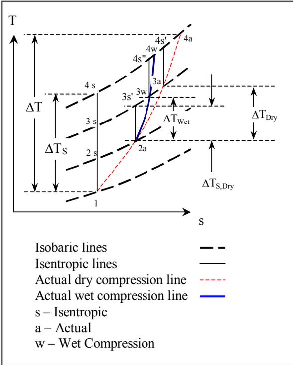
**Figure 1 Pre-heat and pre-cool effect on air due to evaporative cooling. This figure only qualitatively represents the behavior of the air, but not the complete wet compression process.**
