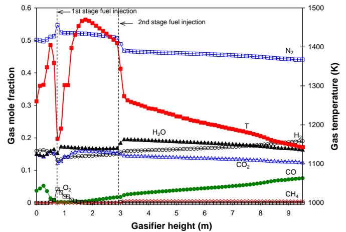
Fig. 12 Mass-weighted averages of gas temperature and species mole fraction distributions along gasifier height for Case 5 (2-stage, 75%-25%, coal slurry, air-blown).
