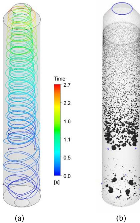
Fig. 6 (a) Flow pathline colored by the residence time temperature and (b) particle distribution for Case 1.
