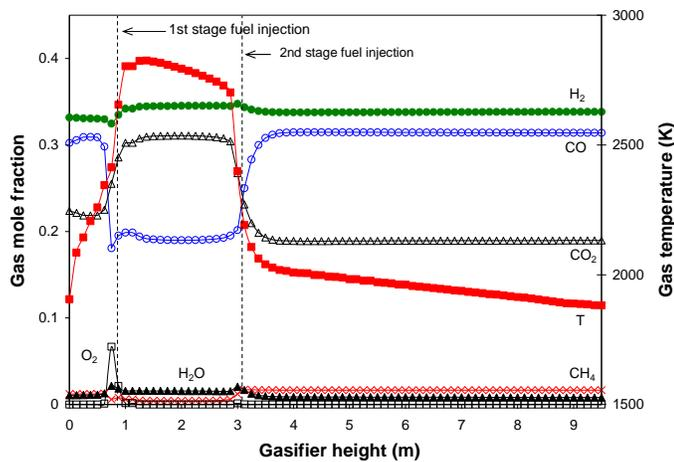
**Fig. 9 Mass-weighted averages of gas temperature and species mole fraction distributions along gasifier height for Case 2 (2-stage, 75%-25%, dry coal, oxygen-blown).**
