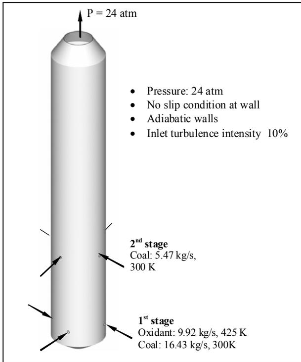
Fig. 3 Boundary conditions of the baseline case of the two-stage entrained-flow gasifier.
