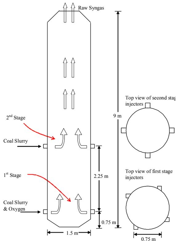
Fig. 1 Schematic of the two-stage entrained-flow gasifier.
