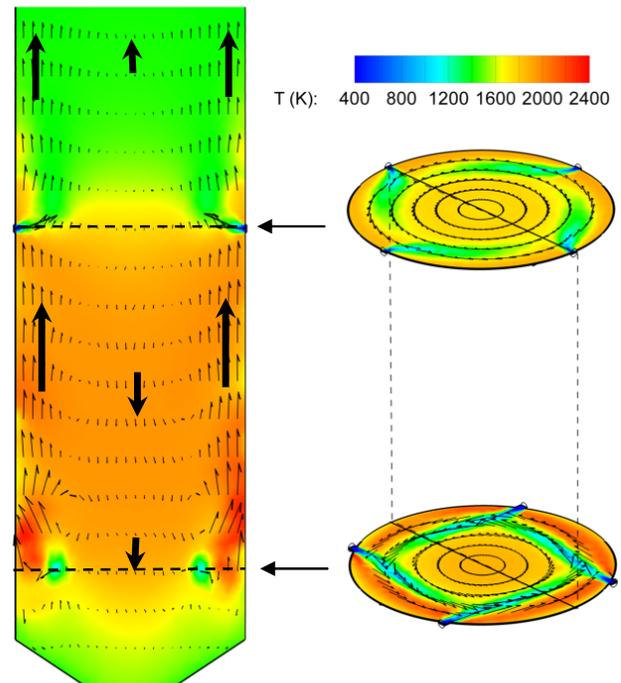
Fig. 7 Velocity vectors and temperature field on the center vertical plane and injection planes for Case 1.
