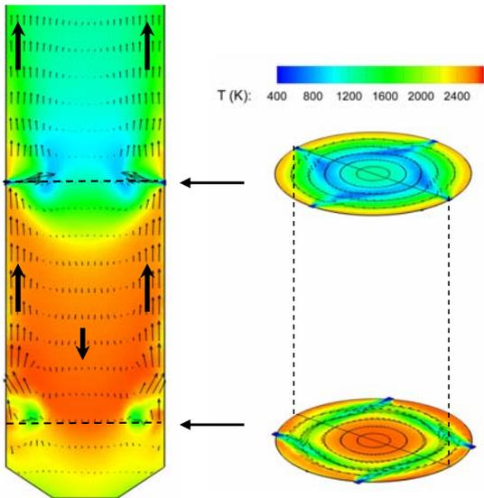
Fig. 11 Velocity vectors and temperature field on the center vertical plane and injection planes for Case 3 (50%-50%).
