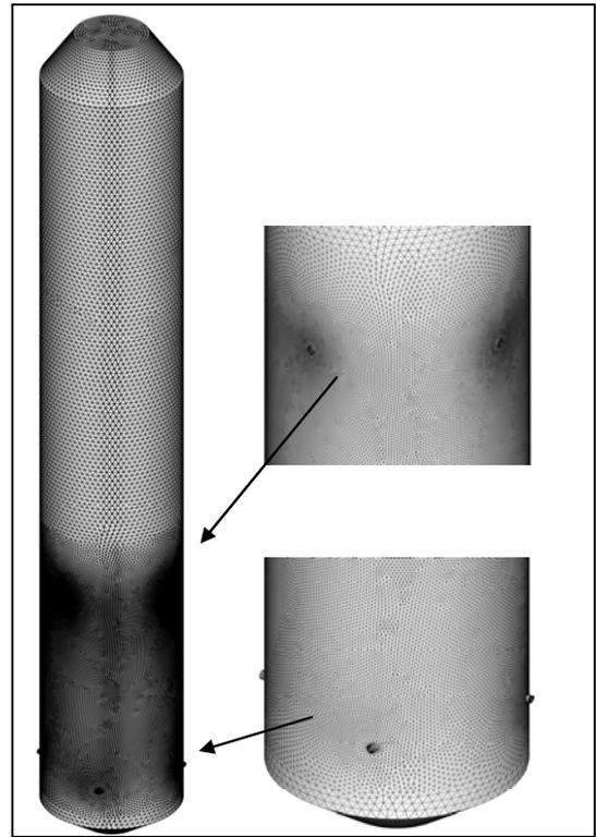
Fig. 2 Meshed computational domain of the two-stage entrained-flow gasifier.
