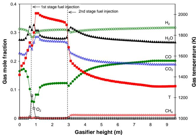
**Fig. 5 Mass-weighted averages of gas temperature and species mole fraction distributions along gasifier height for Case 1 (2-stage, 75%-25%, coal slurry, oxygen-blown).**
