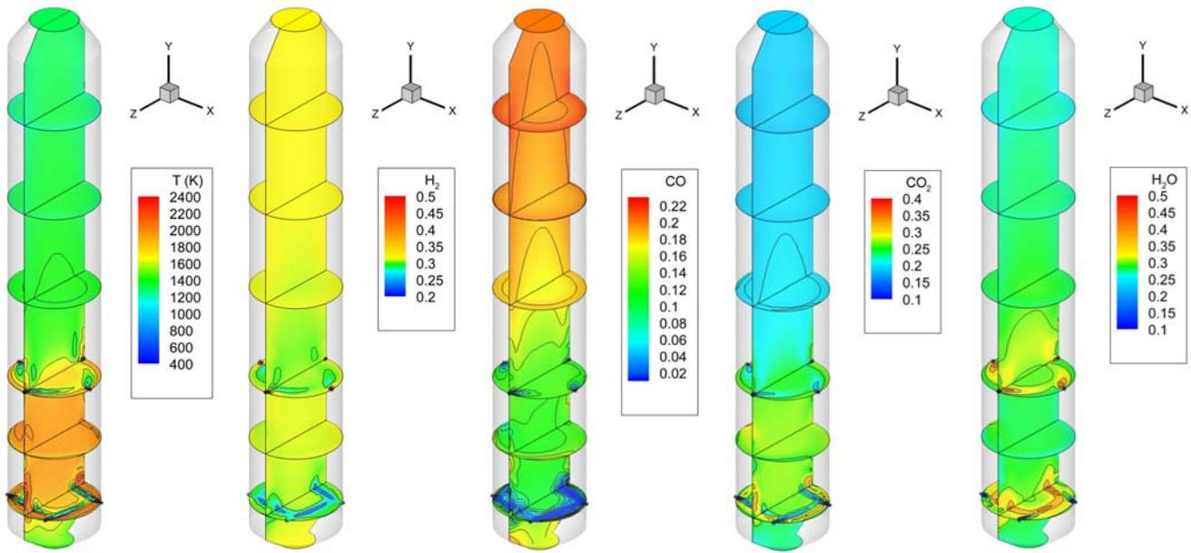
**Fig. 4 Gas temperature and species mole fraction distributions for Case 1 (2-stage, 75%-25%, coal slurry, oxygen-blown).**
