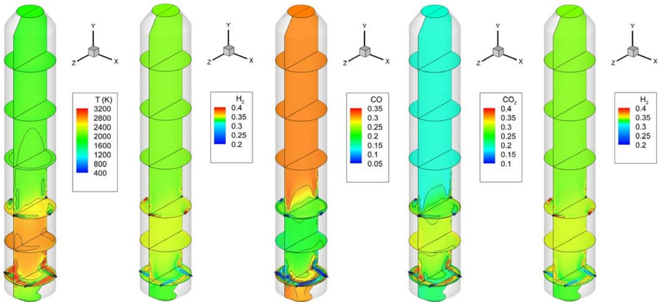
**Fig. 8 Gas temperature and species mole fraction distributions for Case 2 (2-stage, 75%-25%, dry coal, oxygen-blown).**
