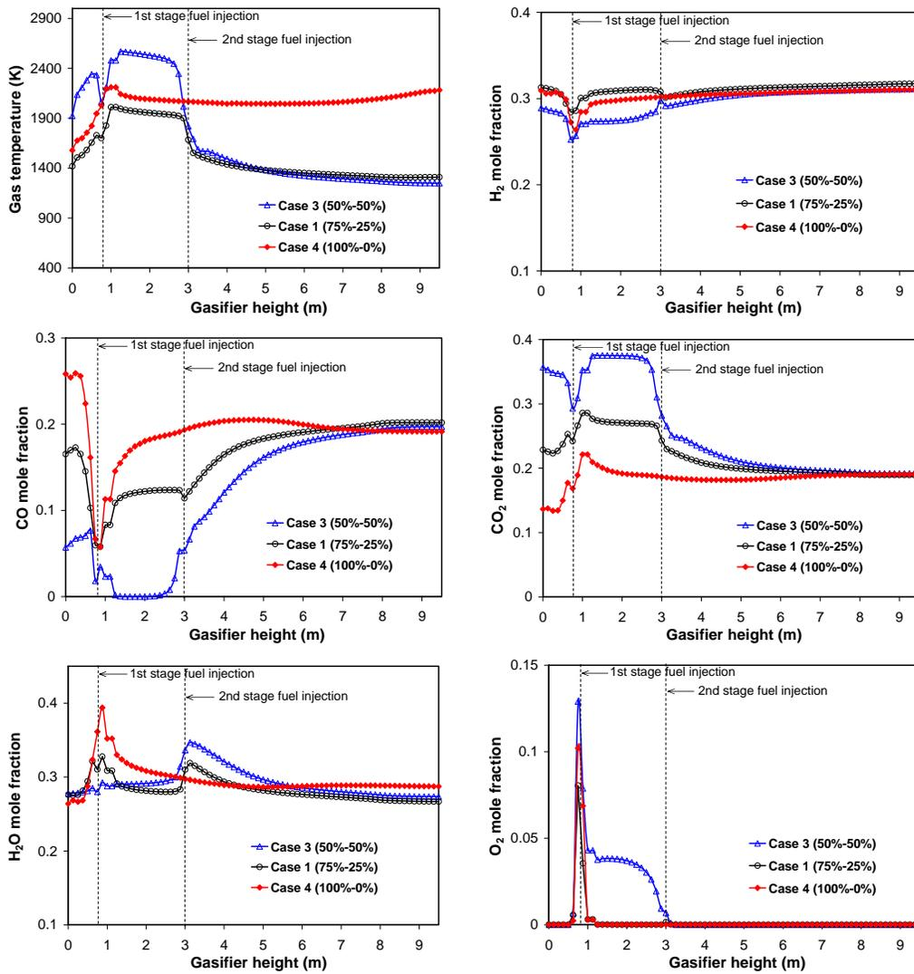
Fig. 10 Mass-weighted averages of gas temperature and species mole fraction distributions along gasifier height for Cases 1, 3 and 4.
