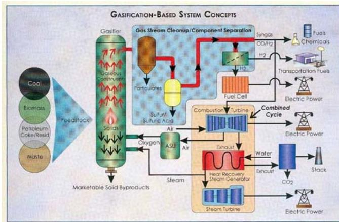
Figure 1 Typical IGCC plant using biomass feedstock (Source: U.S. Department of Energy)
