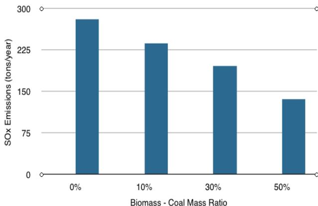
Figure 9 SO<sub>x</sub> emissions for various amounts of biomass blending
