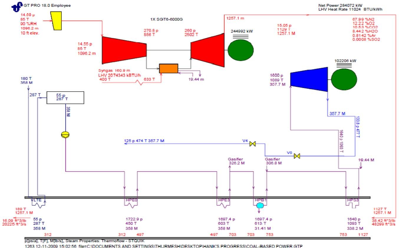
Figure 4 Pure coal (0% biomass) plant power block specifics
