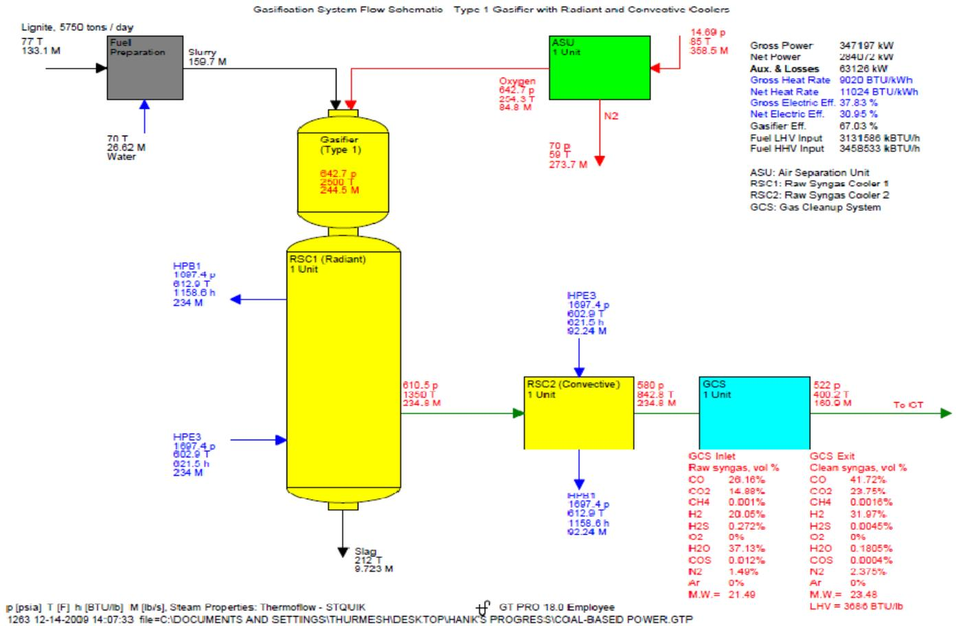
Figure 3 The slurry-fed, oxygen-blown, entrained-flow gasifier design layout
