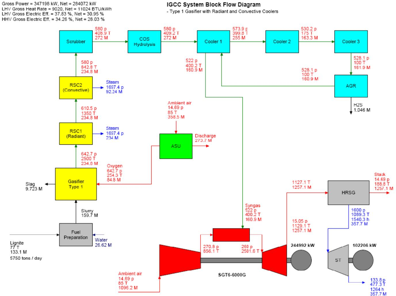
Figure 2 IGCC baseline plant design. Parameters in the figure: P (psia), T (°F), h (Btu/lb), M (lb/s).
