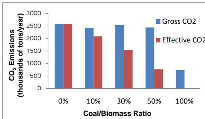
**Figure 6 Gross and effective CO<sub>2</sub> emissions for various amounts of biomass blending**
