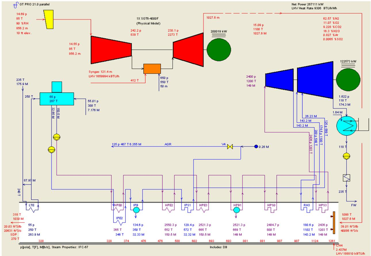
Figure 3 System Design (0% biomass, supercritical steam cycle case)
