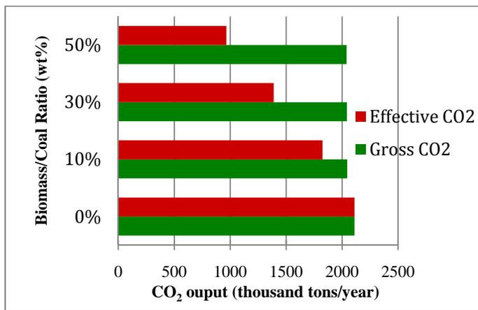
Figure 9 CO<sub>2</sub> output for various amounts of biomass (subcritical only)
