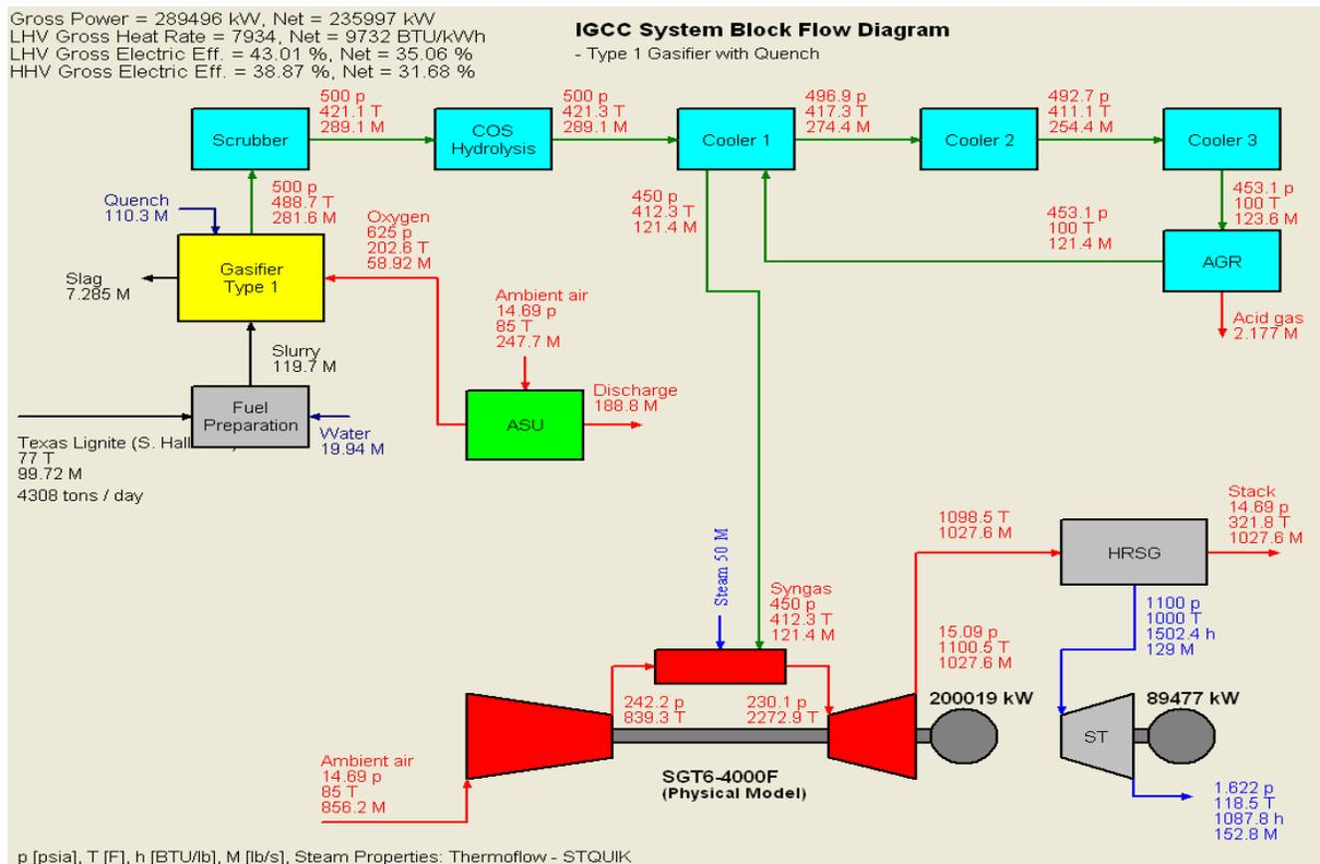
Figure 4 IGCC overall plant layout (0% biomass, subcritical steam cycle case)
