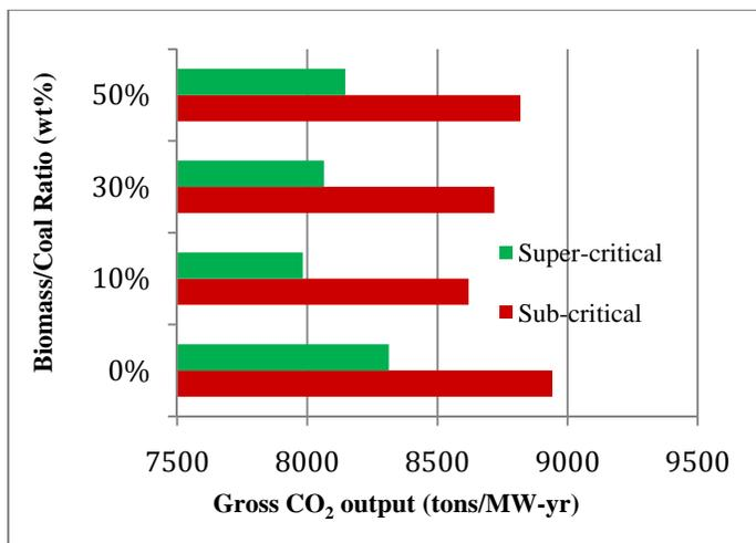
Figure 10 Gross CO<sub>2</sub> output for various amounts of biomass, per MW basis.
