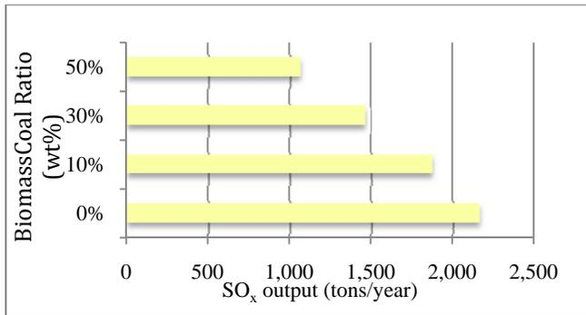
Figure 8 SO<sub>x</sub> emissions data for various amounts of biomass (both plants nearly identical)
