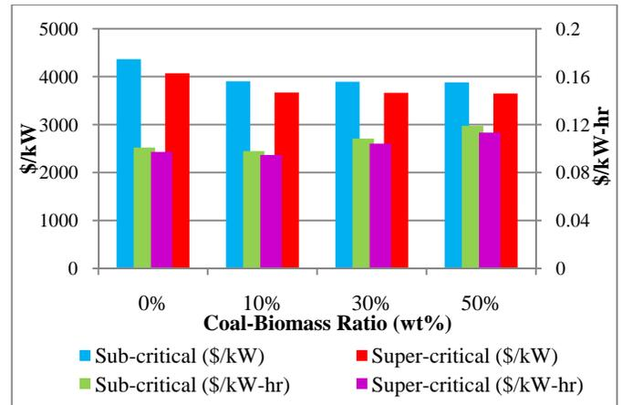
Figure 11 Average costs for sub- and supercritical IGCC cycles with varying amounts of biomass.
