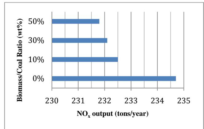
**Figure 7 NO<sub>x</sub> emissions for various amounts of biomass blending (both plants nearly identical)**
