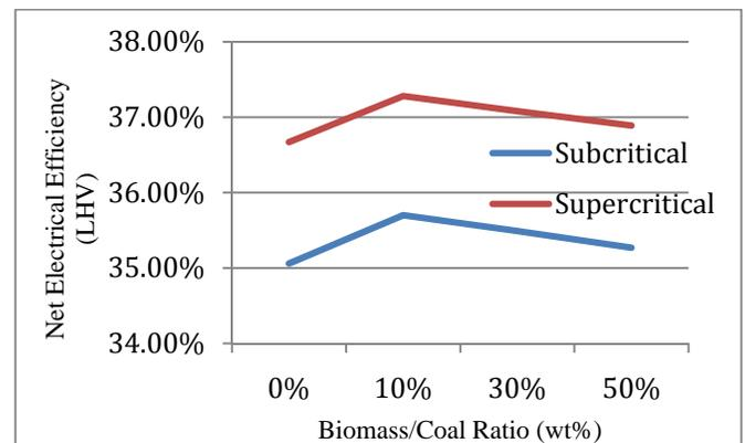
**Figure 6 Net efficiency for various amounts of biomass**
