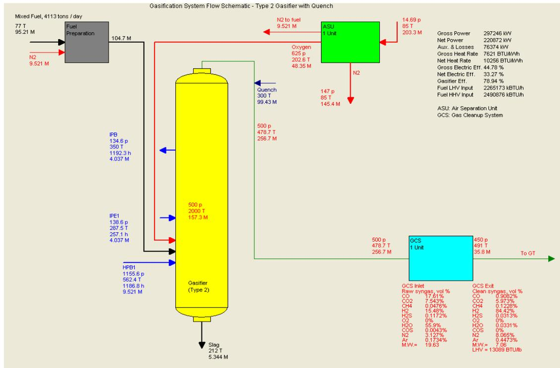
Figure 3 Dry-fed gasification system [P(psia), T(F), h (Btu/lb), m (lb/s), q (Btu/s)]
