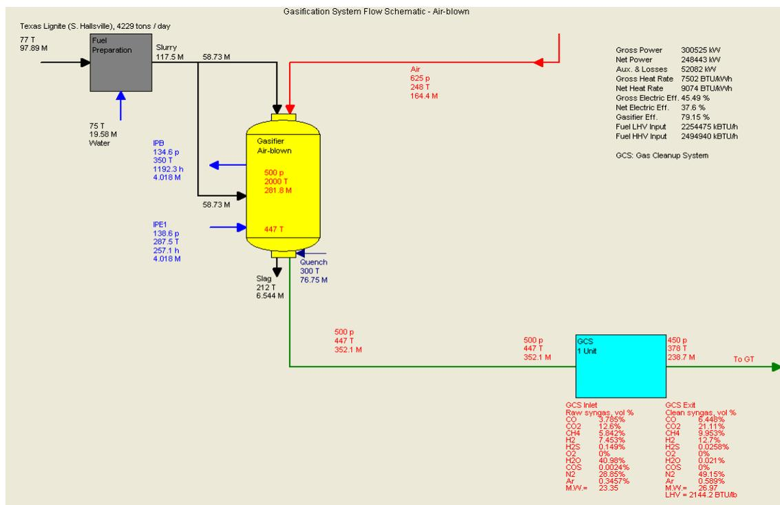
Figure 4 Air-blown gasification system
