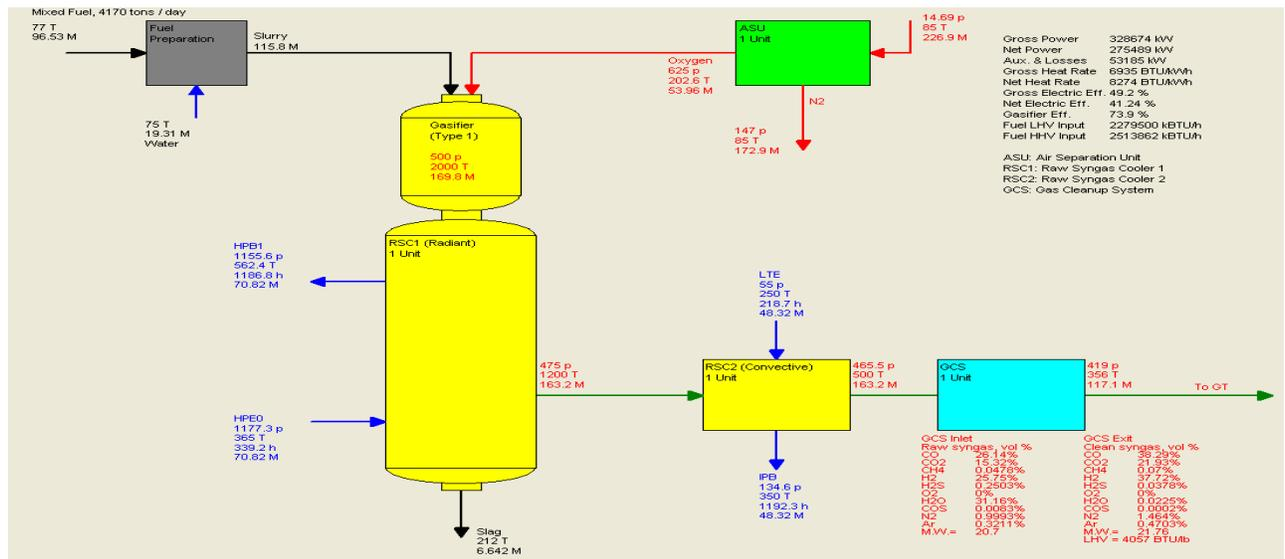
Figure 2 Quench system (top) vs. Radiant and convective coolers (bottom)
