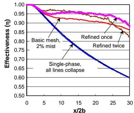
Figure 5 Cooling effectiveness with different grid systems
