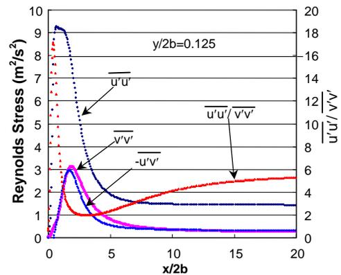
Figure 10 Reynolds stresses predicted by the RSM model
