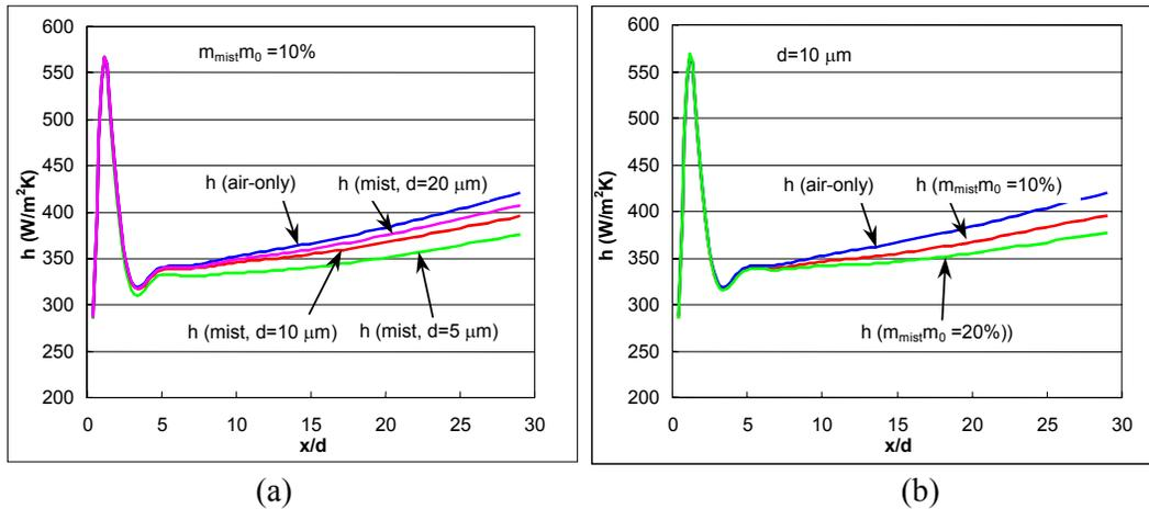
Figure 6 Effects of (a) droplet size and (b) mist concentration on film cooling with the compound-angle diffuse hole over a uniformly cooled base wall under GT operating condition (15atm and 1561K).
