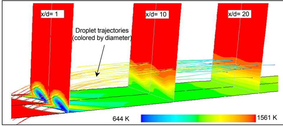
Figure 3 Temperature field and droplet trajectories with the 3-D compound-angle hole.
