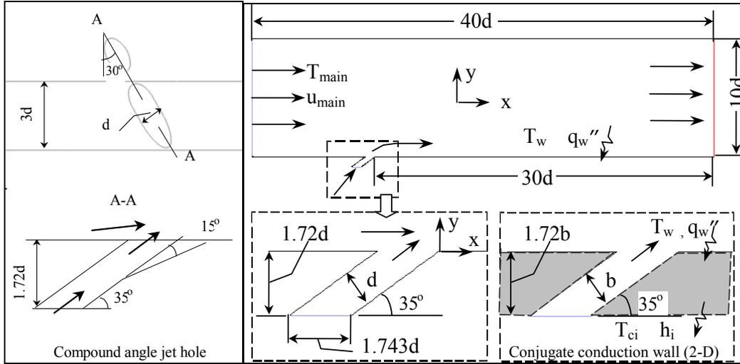
Figure 1 Computational domain and cooling hole configurations
