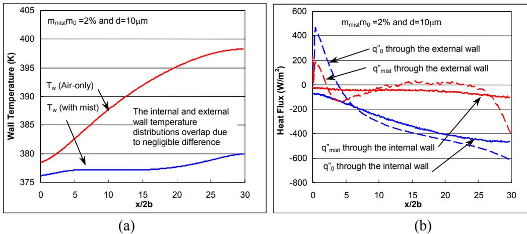
Figure 9 Heat transfer result of mist film cooling of a 2-D slot jet with a conjugated wall cooling.
