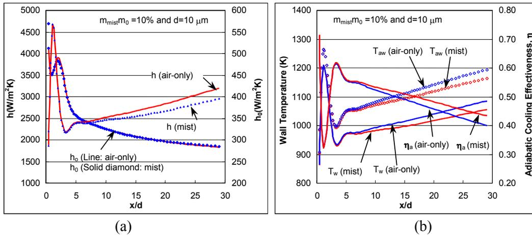
Figure 5 Heat transfer results of the 3-D case with the compound-angle hole over a uniformly cooled base wall under GT operating condition (15atm and 1561K)
