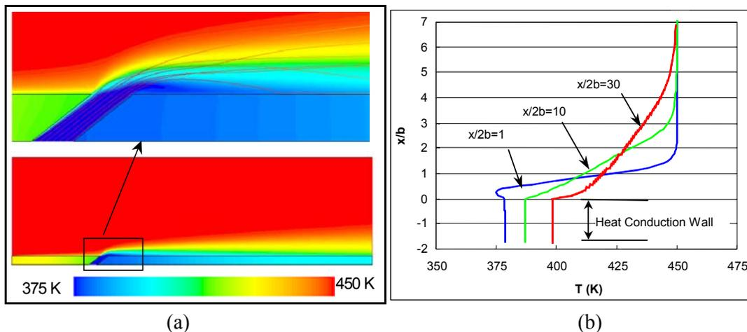
Figure 8 Temperature distribution of 2-D film cooling with conjugate heat transfer
