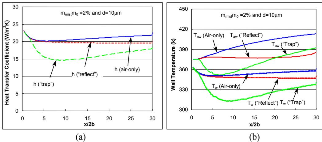
Figure 7 Heat transfer result of the 2-D slot case at low operational conditions (1 atm and 450K).
