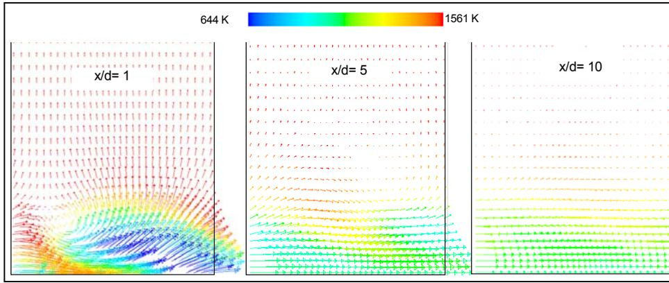
Figure 4 Flow field on planes perpendicular to the mainstream direction for 3-D compound-angle hole case (Colored by temperature)
