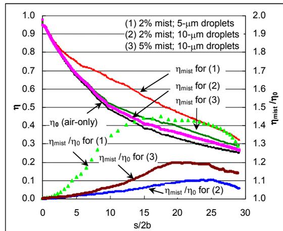
Figure 7 Effects of the droplet size and mist concentration on film cooling enhancement at the leading edge
