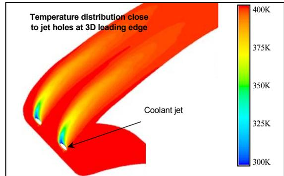
Figure 15 Temperature distribution of air film cooling on 3-D leading edge surface
