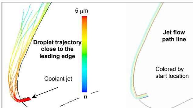
Figure 5 Droplet Trajectories vs. jet flow pathlines for Leading Edge Mist Cooling
