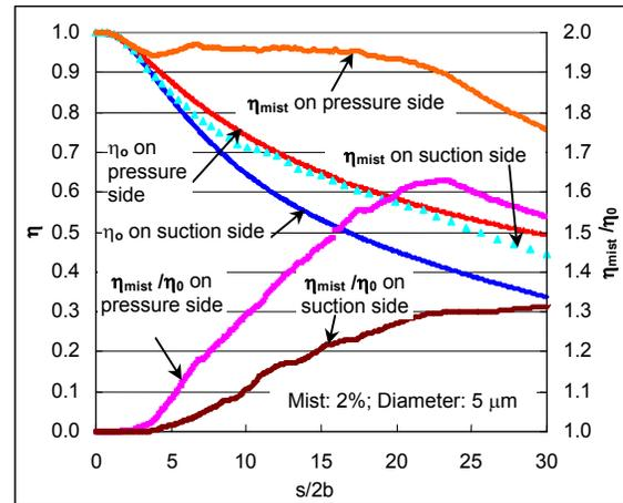
Figure 13 Enhancement of film cooling with mist injection on concave and convex surfaces.
