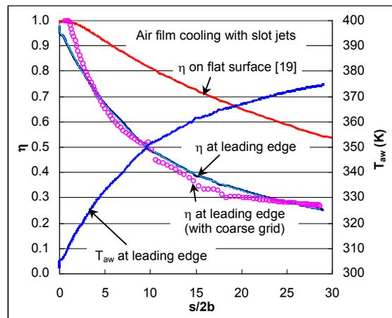
Figure 4 Comparison of air-only leading-edge adiabatic cooling effectiveness with that on a flat surface with the same nominal blowing ratio of 1.33.
