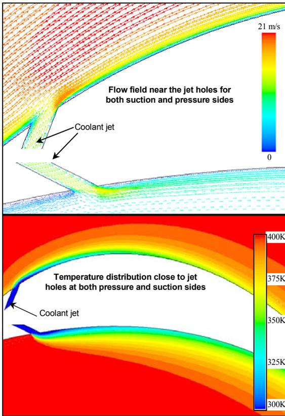
Figure 11 Flow pattern and temperature distribution of film cooling under the curvature effect on pressure and suction sides.
