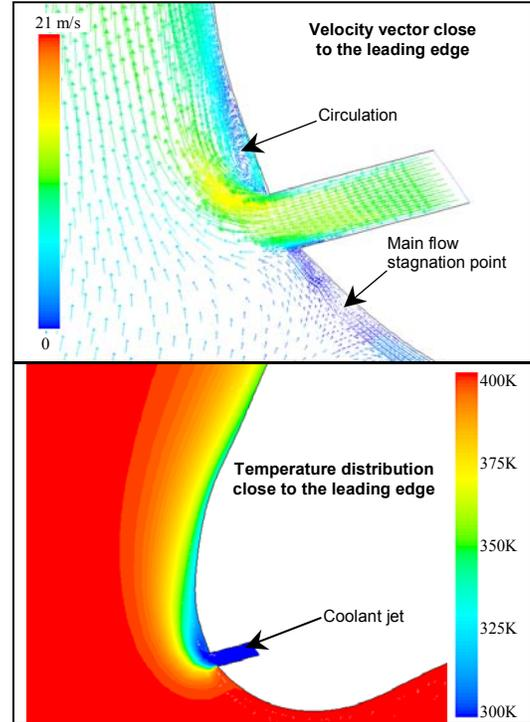
Figure 3 Flow pattern and temperature distribution
