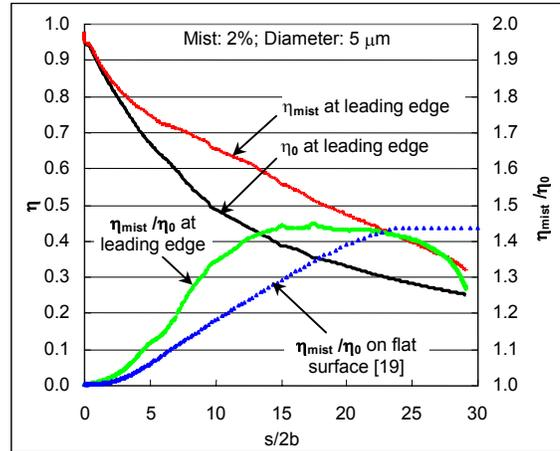
Figure 6 Enhancement of adiabatic cooling effectiveness by injecting mist with the nominal blowing ratio of 1.33
