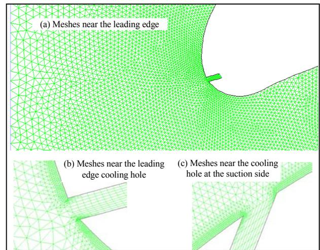
Figure 2 Meshes of partial domain and details near Injection holes (with grid adaptation)
