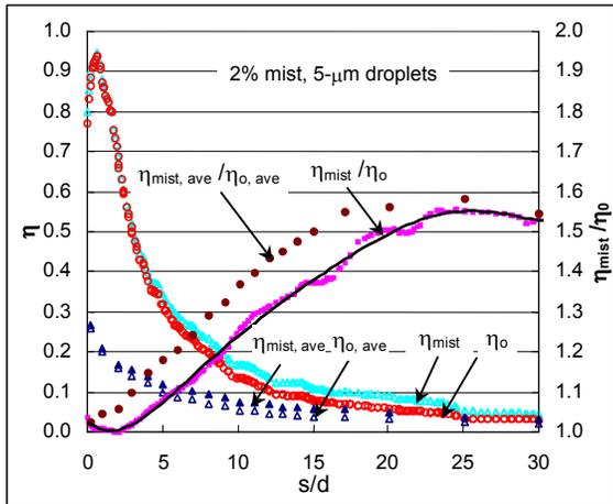
Figure 16 Adiabatic cooling effectiveness of 3D leading edge film cooling and its enhancement with mist injection
