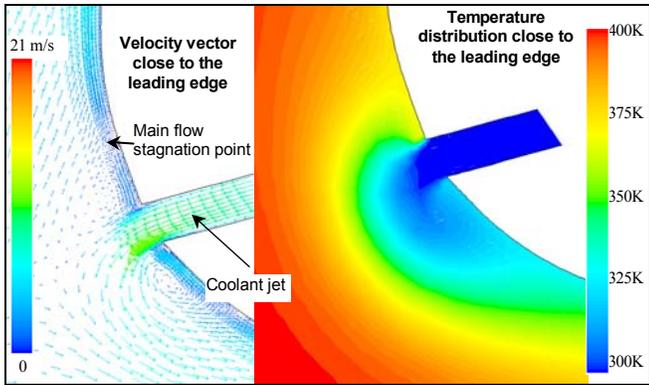
Figure 8 Effect of the main flow incident angle on flow and temperature distribution close to the leading edge
