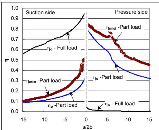
Figure 9 Effect of the main flow incident angle on adiabatic film cooling effectiveness near the leading edge.
