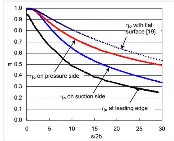
Figure 12 Comparison of air-only film cooling effectiveness on flat and curved surfaces with a nominal blowing ratio of 1.33.
