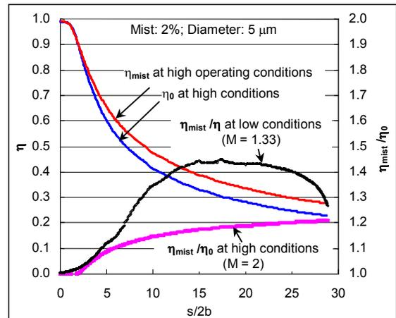
Figure 10 Effect of elevated operating conditions on mist film cooling performance of the turbine blade leading edge
