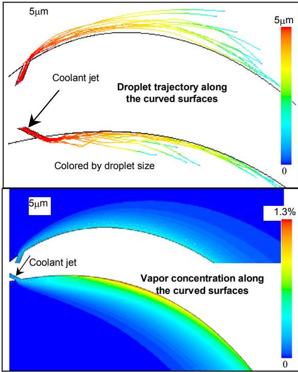
Figure 14 2-D droplet trajectories and vapor concentration in mist film cooling with concave and convex surfaces.
