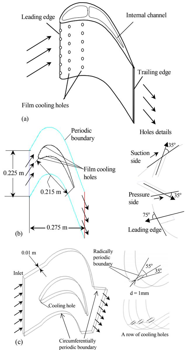
Figure 1 Schematic of film cooling and computational domain (a) film cooling concept (b) 2-D cases (c) 3-D cases
