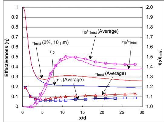
Figure 8 Centerline and spanwise average cooling effectiveness and mist cooling enhancement (round-hole)
