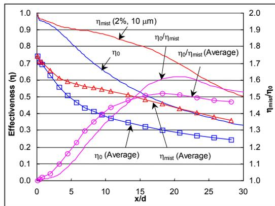
Figure 9 Centerline and spanwise average cooling effectiveness and mist cooling enhancement (fan-shaped hole)
