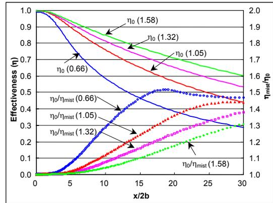
Figure 16 Effect of mist injection on the slot jet air film cooling with different blowing ratios
