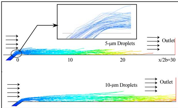
Figure 15 Droplet trajectories predicted with stochastic tracking (2-D slot case)
