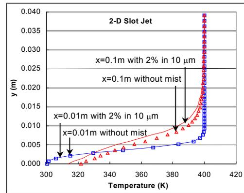
Figure 5 Effect of 2% mist injection on temperature distribution at different locations (Slot jet)
