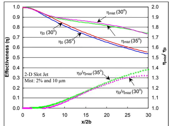
Figure 17 Effect of mist injection on the slot-jet air film cooling with different blowing angles
