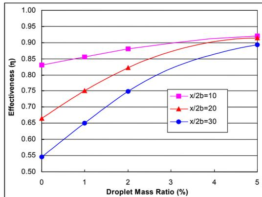
Figure 13 Effect of mist concentration on cooling effectiveness for a 2-D slot film cooling
