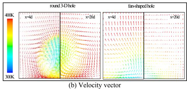
Figure 10 Cross-sectional temperature distributions and velocity fields in the streamwise direction (Film cooling without mist).
