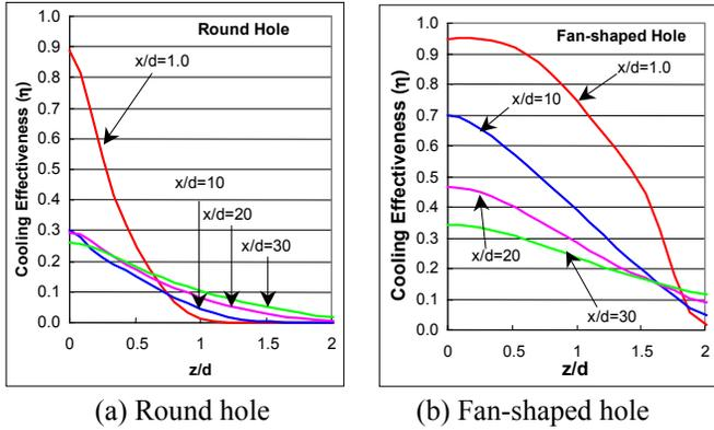
Figure 11 Spanwise distributions of cooling effectiveness for round and fan-shaped holes (Film cooling without mist).
