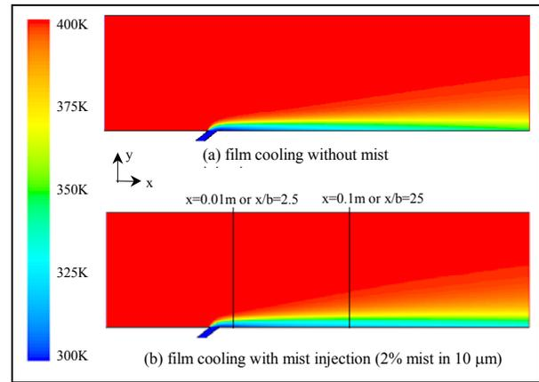
Figure 4 Temperature distribution of air-film cooling with and without mist injection (Slot jet)
