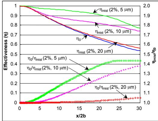
Figure 14 Effect of droplet size on cooling effectiveness for a 2-D slot film cooling.
