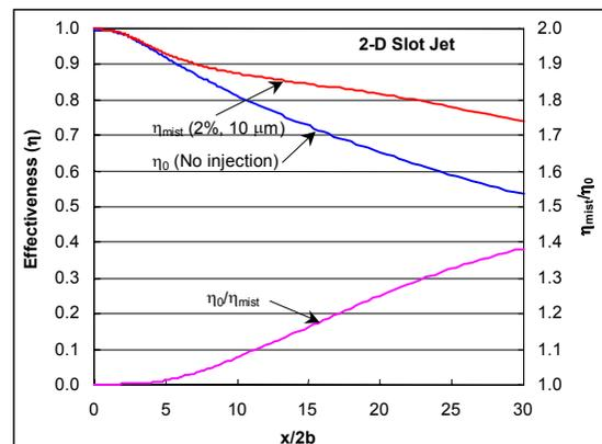
Figure 6 Effectiveness of film cooling and mist enhancement (2-D slot)
