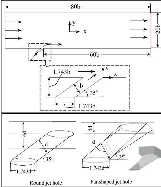
Figure 1 Computational Domain and Film Hole Configurations
