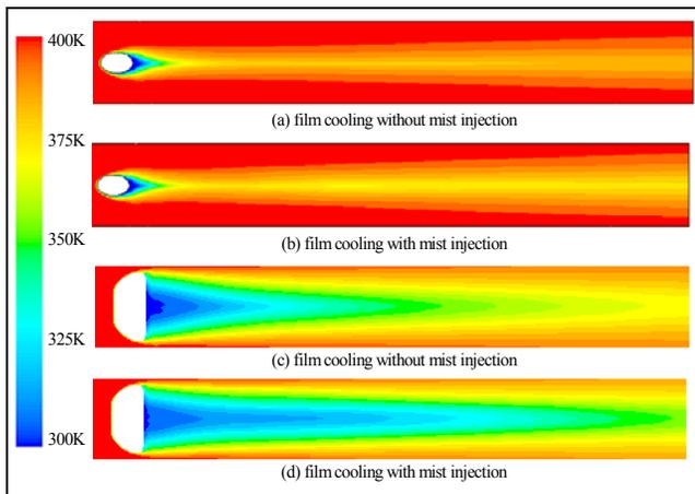
Figure 7 Wall temperature distributions of air-film cooling on the cooling surface for both round and fan-shaped holes.
