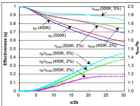
Figure 18 Effect of mist film cooling with different mainstream temperatures
