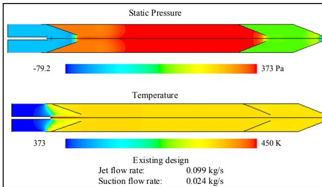
**Figure 3: Pressure and temperature fields of the existing design**
