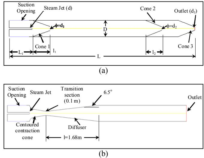
**Figure 1: Geometric scheme of (a) the existing design and (b) the case with best performance**
