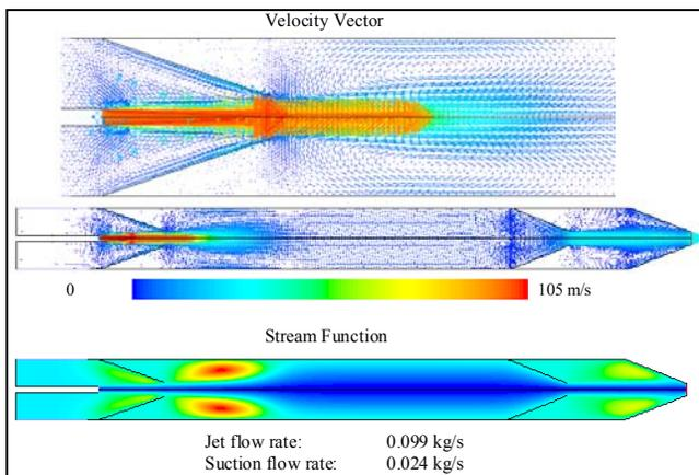
**Figure 4: Velocity field and stream function of the existing design**
