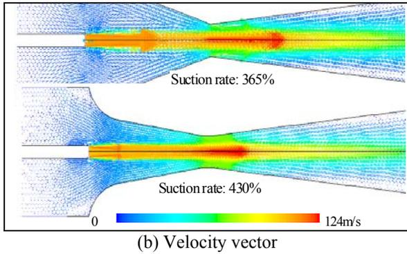
**Figure 8: Effect of the contraction cone contour on the ejector performance**
