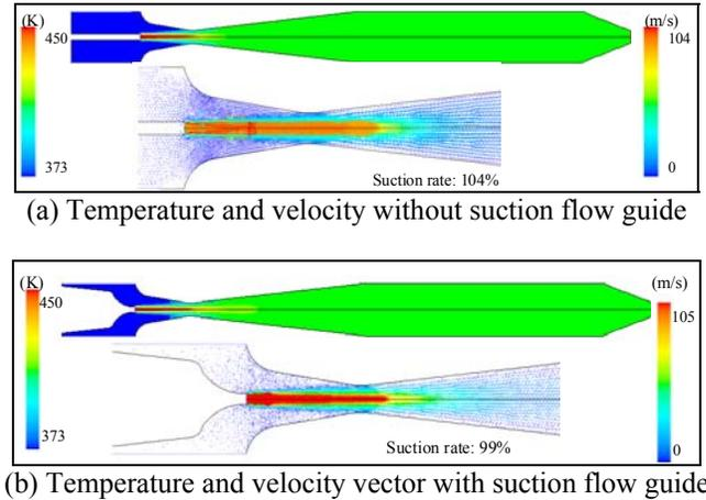
**Figure 10: Comparison of the ejector performance with and without suction flow guide**
