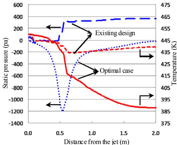
**Figure 12: Temperature and pressure distributions along the ejector centerline in different cases**
