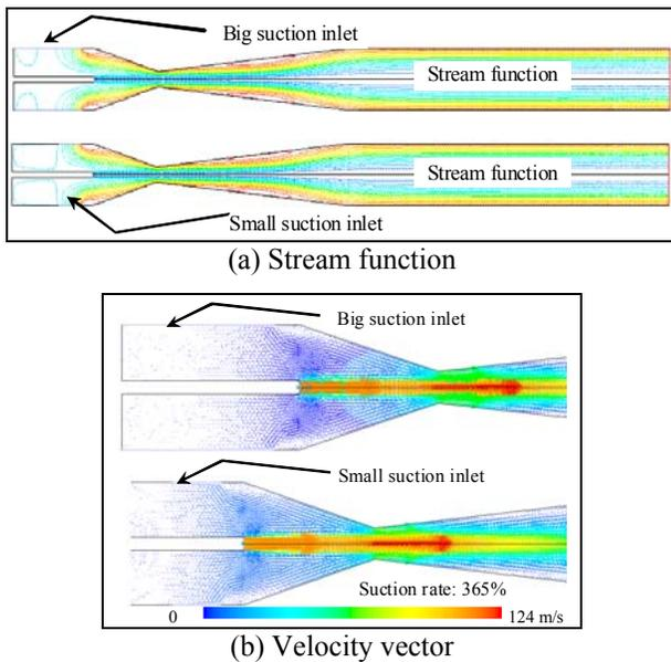
**Figure 9: Effect of the suction opening size**
