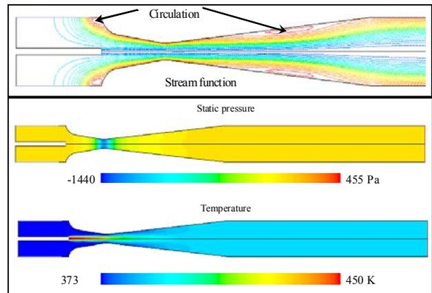
**Figure 11: Flow pattern and temperature distribution for the optimized ejector case**
