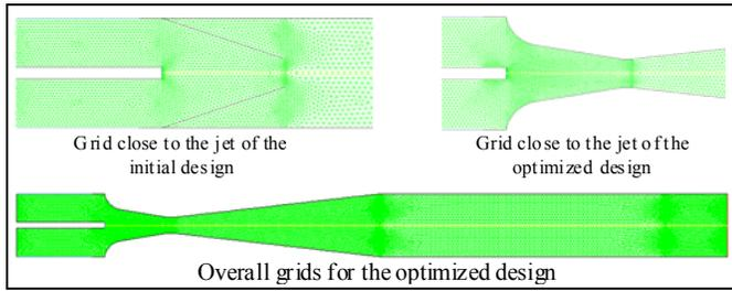
**Figure 2: Computational meshes for different cases**
