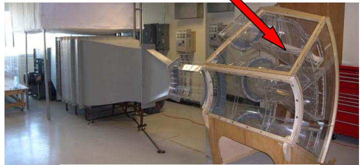
1/7th sector of dump diffuser-combustor
