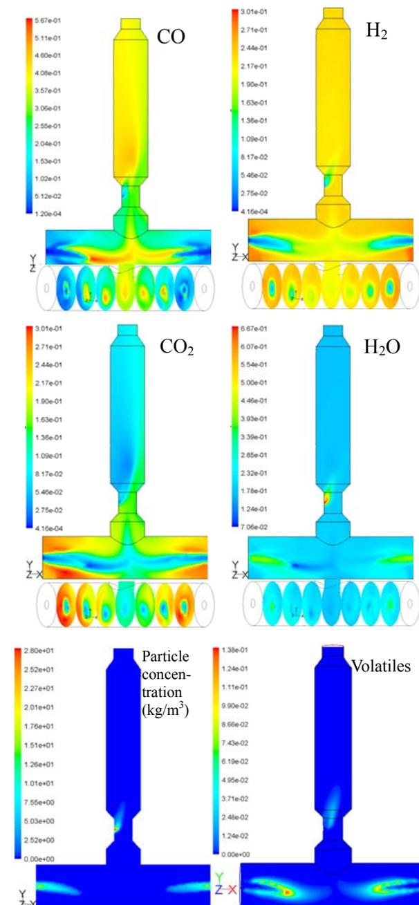
Fig. 3 Species mole fraction contour, particle concentration, and volatiles contour of base case
