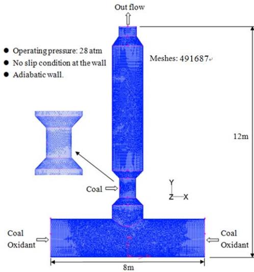
Fig. 1 Schematic of computational model
