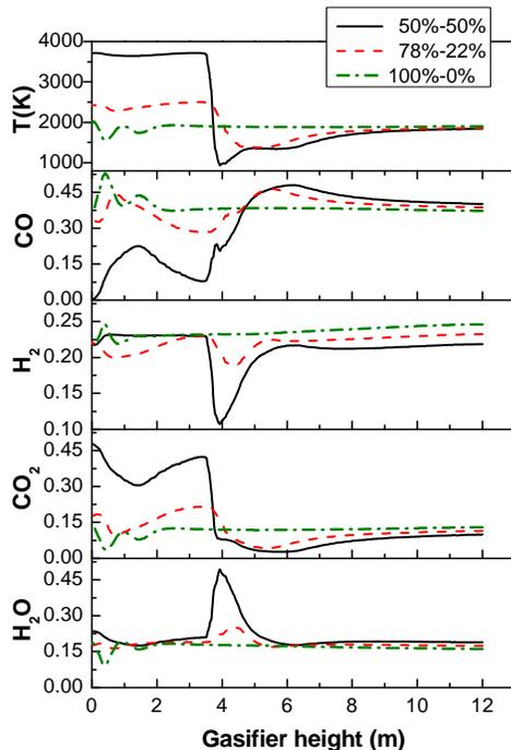
Fig. 5 Mass-weighted temperature and mole fraction distributions along the gasifier height on different fuel distribution conditions
