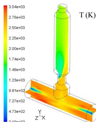
Fig. 2 Temperature contours of the base case
