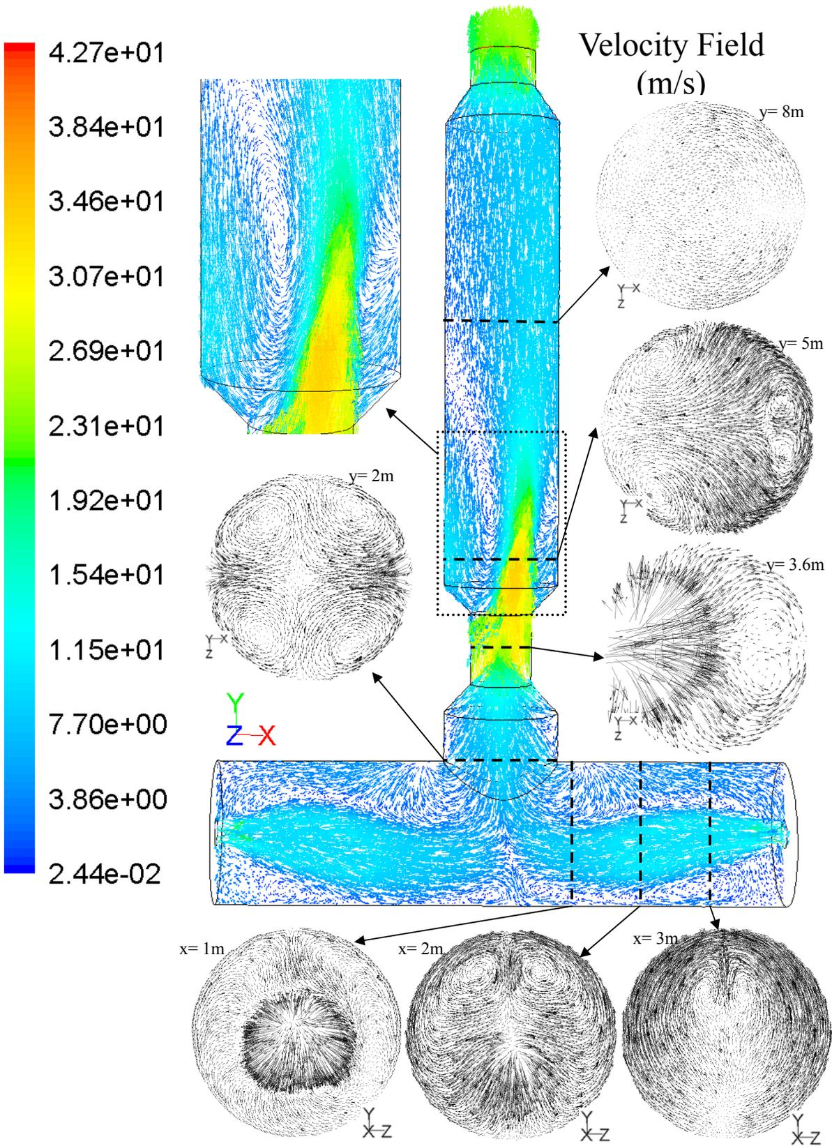
Fig. 4 Velocity vector of xy-plane and cross-section plane at different positions
